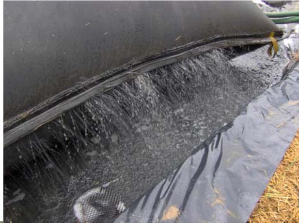
This bag was opened approx 2 weeks after the last pumping. The sludge shown is a municipal waste water sludge. The flocculation process was very well controlled, maximum dewatering allowed these solids to be handled very quickly. Results may vary depending on how well the material is flocculated and the process controlled. Most bags are left to dewater for periods of from 2 months to 12 months depending on available space and time.
