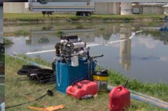
This 24 hp hydraulic unit is used to power the submersible pump on the pumping raft.
