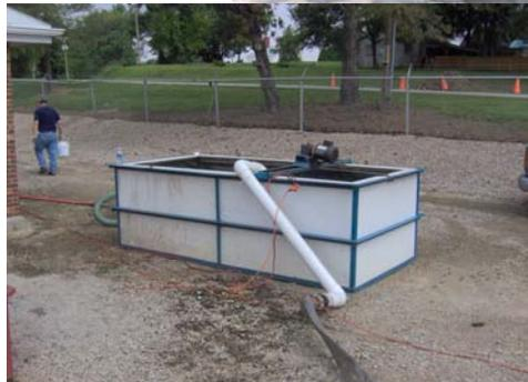
This 24 hp hydraulic unit is used to power the submersible pump on the pumping raft.
