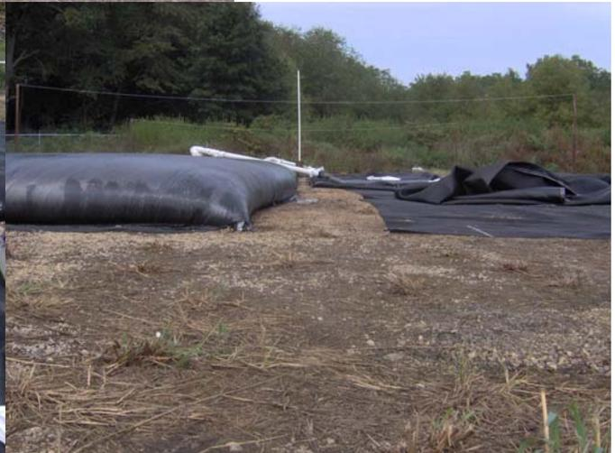
As the bags are filled the clean effluent flows out of the bag and back to the plant. The digester slowly begins to draw down.
